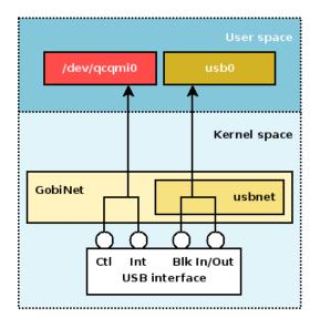
Figure 1: GobiNet in the Linux kernel
